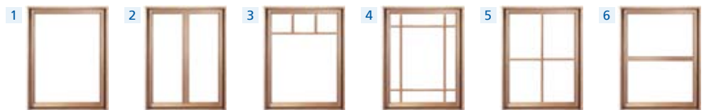
1 Standard 2 Simulated Casement or Georgian Bar 3 Heritage Bar 4 Federation Bar 5 Colonial Bar 6 Simulated Double Hung
